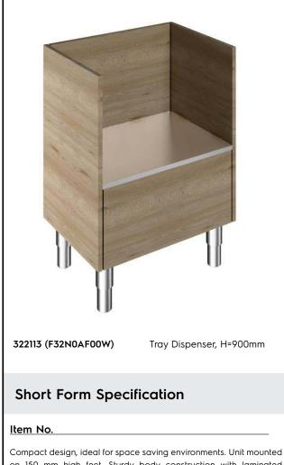
Compact design, ideal for space saving environments. Unit mounted on 150 mm high feet. Sturdy body construction with laminated panelings on 4 sides. 900mm worktop height. Tray dispenser, designed to hold trays, towels, cutlery dispenser and the bread dispenser.
